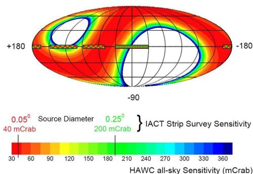
Figure 3: Flux limits for HAWC versus the HESS sky survey and the proposed VERITAS sky survey over the next two years. HAWC is assumed to be located in Mexico ( $19^\circ$ N). IACT sensitivity is shown for point (red) sources and for sources extended by  $0.25^\circ$  (green). A crab-like spectrum is assumed. The HAWC limits will be lower for harder sources.
