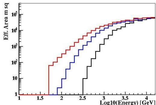
Figure 2: HAWC effective area versus gamma-ray energy for three different levels of trigger multiplicity (20(upper red line), 80(blue line) and 200(lower black line) PMT trigger) for a zenith angle  $< 30^\circ$  after applying the cosmic ray background rejection cut and requiring a reconstructed direction within  $1^\circ$
