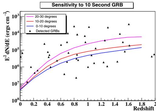
Figure 2: HAWC Sensitivity to a 10 second GRB. The lines are for GRBs at different zenith angles & the triangles are observed GRBs with known redshifts. It can be seen that HAWC has the potential to detect approximately half the GRBs in its field of view if their spectra extend above  $\sim 300$  GeV
