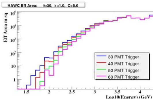
Figure 1: HAWC effective area for gamma-rays. This is for showers within 30° of zenith, passing the gamma-hadron cut, which reconstruct within 1° of the true angle. For a 30 pmt trigger HAWC will have nearly 70m<sup>2</sup> at 100 GeV and 10<sup>4</sup>m<sup>2</sup> at 1 TeV.
